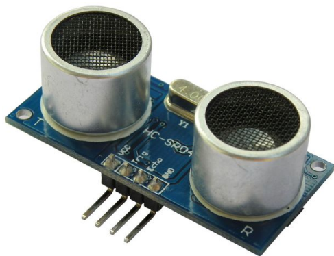
(a) Ultrasonic module HC-SR04;
